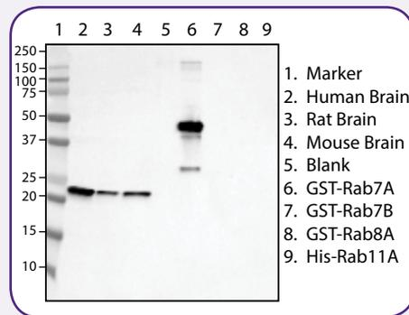
Western blot of purified anti-Rab7A antibody (clone W16034A). M: Molecular weight marker; brain lysates: 20 µg; recombinant proteins: 10 ng.
