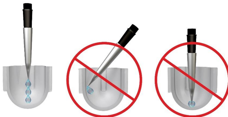
Figure 8. When loading cells and beads into the Quantum Barcoding Plate, ensure that you are pipetting dropwise over the center of each well to allow for even distribution across the entire well.
