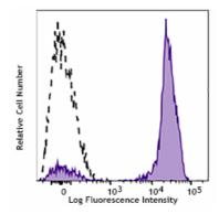
Typical results from human peripheral blood lymphocytes stained either with TS1/8 PE/Cyanine7 used at 5 µL/test (filled histogram) or with an isotype control (open histogram).
